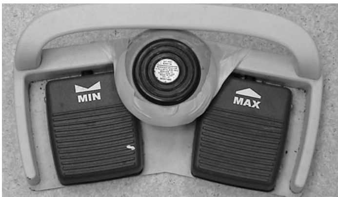
Figure 5 – Foot pedal configuration for simultaneous use of the bipolar electrocautery and the harmonic scalpel (Bipolar pedal is taped to a ridge on the harmonic scalpel pedal so the pedals remain fixed in place).
